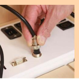
Connect the circular connector to power supply box. Align the groove in connector to properly insert. Thread the cuff of connector on fully.
