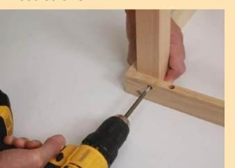
Ensure that the legs' ends are flush with the bottom edge of the frames
