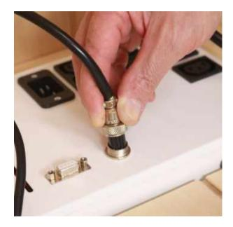
Connect the circular connector to power supply box. Align the groove in connector to properly insert. Thread the cuff of the connector on fully.
