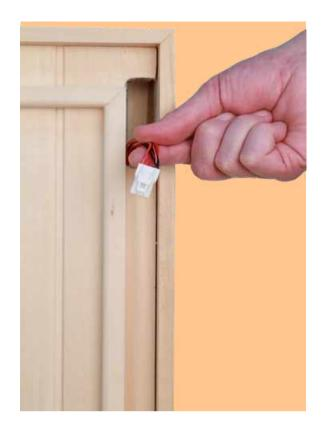
Pull the single plastic connector down and out of the roof before lifting the roof into place. If you are unable to grab hold of the connector through the small opening in the ceiling, it may be necessary to remove the first T&G board on the top left side of the roof and feed the connector down through the opening.
